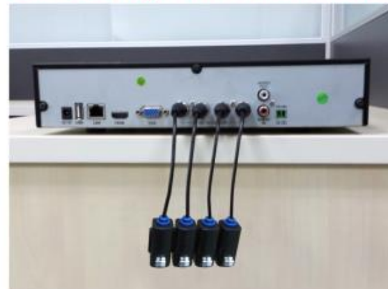
Baluns click together for a neat installation
